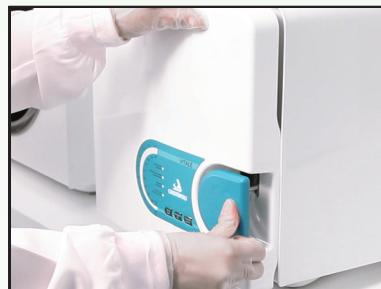
**04** Close the autoclave door and run a sterilization cycle.
