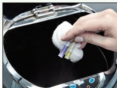
**17** Autoclave the control ampoule wrapped in cotton and autoclave tape in a sterilization envelope (surgical grade paper) and the test ampoule if positive for bacterial growth.
