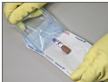
**06** After the sterilization cycle is finished, wait 15 minutes for the packages to cool down. Open the envelope and retrieve the test ampoule that was autoclaved.
