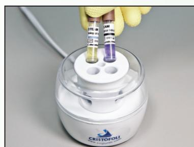
**11** For 24 hours indicators, proceed the initial reading after 8 hours, then 12 hours and the final reading after 24 hours. For 48 hours indicators, proceed also readings after 36 and 48 hours. Note: In case the test ampoule presents the yellow color at any moment, interdict the autoclave immediately and follow the use instructions of the biological indicator manual.
