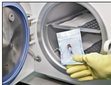
**03** Put one of the biological indicators in an envelope and put the envelope into the autoclave (which already contains a standard load).
