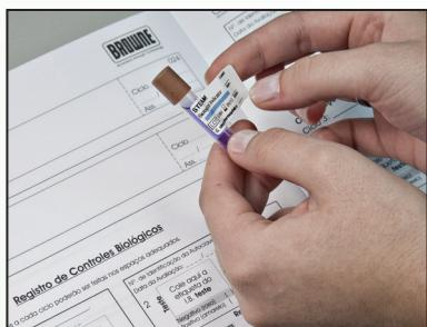
**13** Remove the label from each ampoule (test and control).
