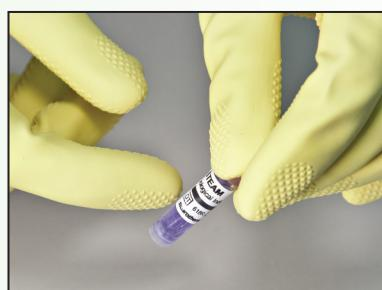
**08** Hold the ampoule as shown. Hit the bottom side of the indicator a few times to make sure the purple growth medium reached the paper disc impregnated with the spores. The upper side of the ampoule has a hydrophobic filter (see photo on page 1), it cannot be wet, do not shake the ampoule.
