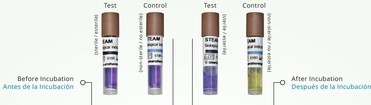
Note that after the sterilization, the chemical indicator of the test ampoule label must have changed from blue to dark gray.
