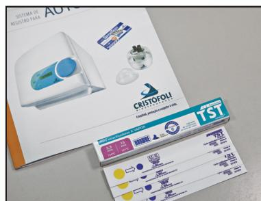
**15** Complement the sterilization monitoring by using at least one chemical indicator (class 6 TST Emulator) on a daily basis. In this case, keep the biological and chemical stickers in the same records book used for the chemical indicators.
