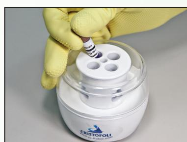
**07** Insert 1/3 of the indicator into the incubator and bend the upper side of the flexible plastic ampoule to activate them. This will crush the internal glass vial, releasing the growth medium to get in contact with the spores. Be careful not to break the external plastic part.
